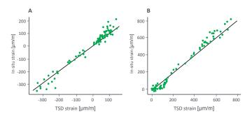
**A.**: In-situ peak transversal strains plotted versus TSD peak transversal strains. The line of equality is shown in black.
