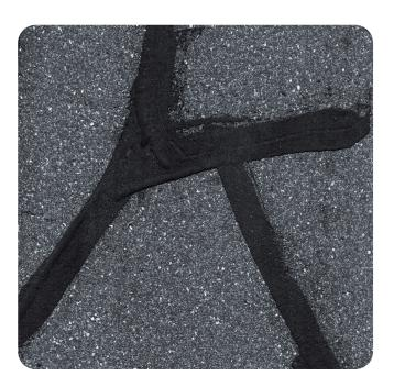
Greenwood's SIS shows the details on the road surface with an unprecedented high image quality. They serve as the best possible foundation for analysis of surface defects, for example with Greenwood's new AI based crack detection algorithm, which scores >94% accuracy on out-sample test set with more than 150 000 images of roads (1.3m x 1m).
