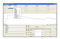
The data acquisition and post processing software handle DGPS information and report information connecting results, time and position. (The GPS NMEA format is standard.) Any relevant algorithm for pavement characteristics can be added. Custom designed filters to obtain national characteristics or indices can easily be built into the modular post processing software.
