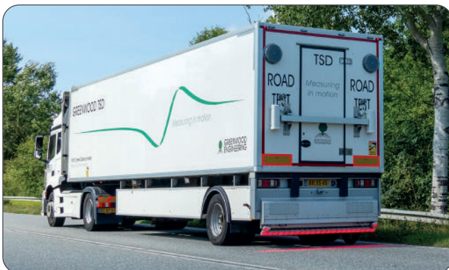
SIS system mounted on the Traffic Speed Deflectometer.
