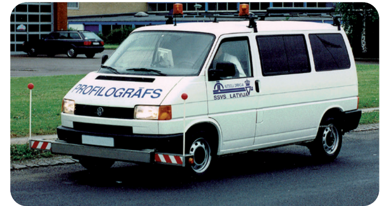
One of the first road profilers with 17 laser and inertial system.
